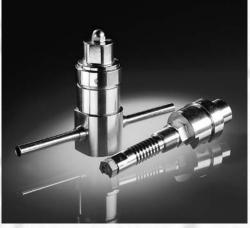
Designed to heat and/or vaporise a gas or liquid sample before entering the analyser system. A steam or electrically heated inlet heat exchanger is utilised to vaporise the sample stream to ensure the flow media stays a gas.
