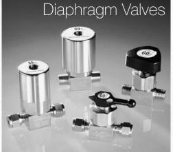
The DV Series Diaphragm Valves are totally free of springs, bellows, packing, o-rings and lubricants in the process wetted area. Metal to metal seals to atmosphere ensure that there is no absorption of undesirable elements into the flow stream. Elgiloy® diaphragms ensure the utmost in corrosion resistance and life span.
